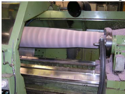
Mandrel Nearing Completion
