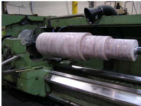
Mandrel Ready for Machining
